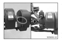
Align the control of the right handlebar half with the markings on the handlebar. Tighten the screws.
