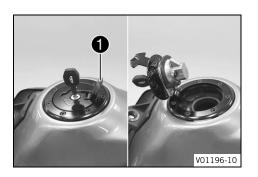
Lift cover **1** of the fuel tank filler cap and insert the ignition key into the lock.
